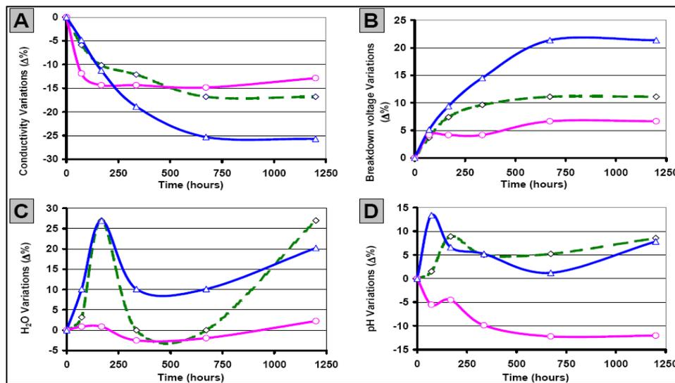
**Figure 1.** Thermal stability test results of the WEY-100 electrolytes, WEY-100-1 (—◇—); WEY-100-2 (—○—); WEY-100-3 (—△—) at 125 °C from 0 to 1200 hours
