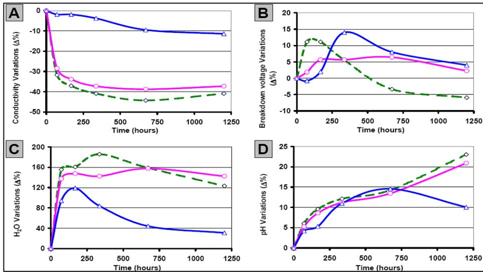
**Figure 2.** Thermal stability test results of the WEY-200 electrolytes, WEY-200-1 (—◇—); WEY-200-2 (—○—); WEY-200-3 (—△—) at 125 °C from 0 to 1200 hours
