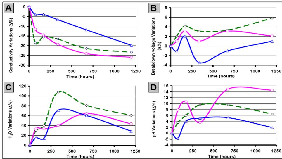
**Figure 3.** Thermal stability test results of the WEY-400 electrolytes, WEY-400-1 (—◇—); WEY-400-2 (—○—); WEY-400-3 (—△—) at 125 °C from 0 to 1200 hours
