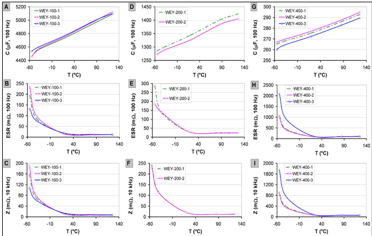
**Figure 4.** Plots of capacitance (C), ESR and impedance (Z) for the 100, 200 and 400 V capacitors as a function of temperature
