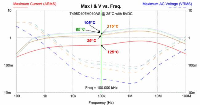
Figure 1. Ta-MnO<sub>2</sub> - Ripple current ( $\Delta T_{max}=20^\circ C$ ) vs. ambient.
