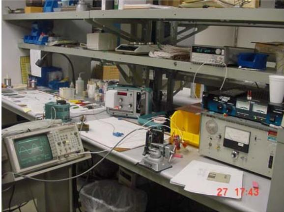
Figure 4. General Overview of the Apparatus for Finding Thermal Resistance from the Capacitor's Core to Terminals.
