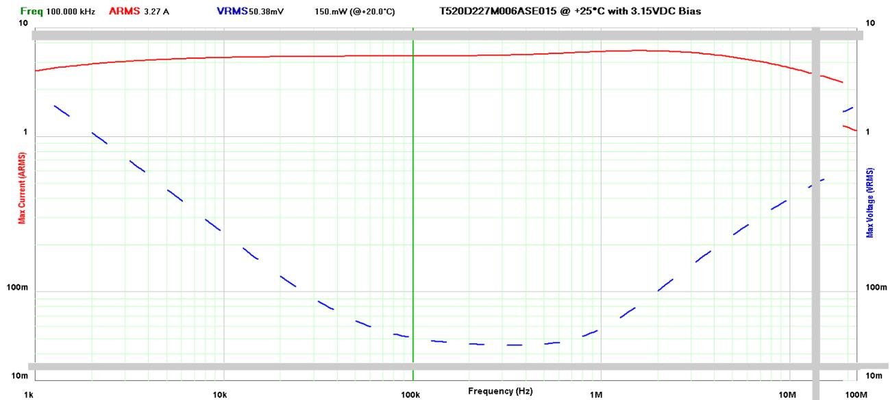
Figure 7. RMS Current & Voltage (truncated) versus frequency (Hz) .
