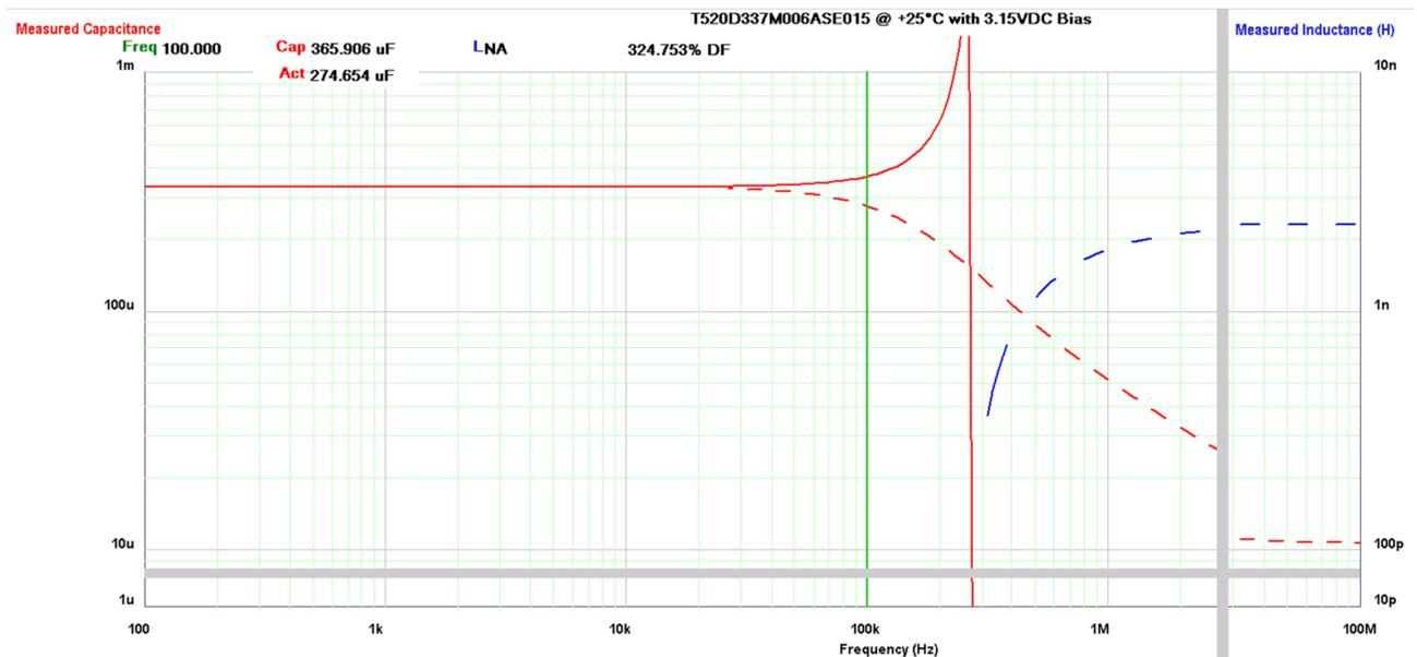
Figure 8. Capacitance drop with frequency for T491 device.
