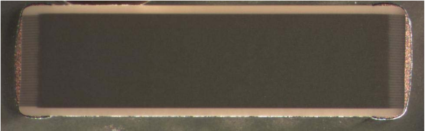
Figure 4. Cross-section of a 2824, 33nF, 630V rated pulse detonator capacitor
