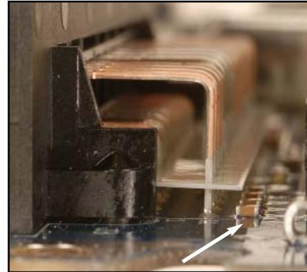
Figure 2. Filter capacitor very near to thru-hole connector.
