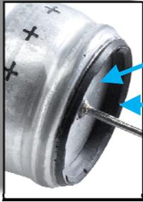
Axial design allows the use of aluminium lid which will not delaminate. The Al-lid is also an efficient diffusion barrier. Specially designed gasket minimizes electrolyte diffusion.
