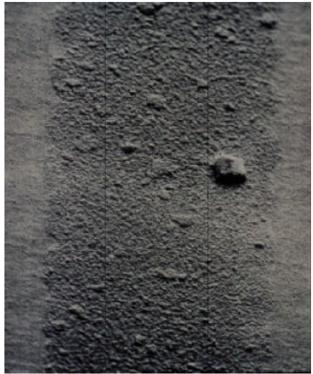
Figure 3a. Traditional internal electrode magnified using SEM
